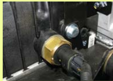
Radiator water level switch
