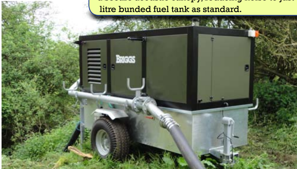
Below: Bunded, acoustic pump; drawbar removed.
